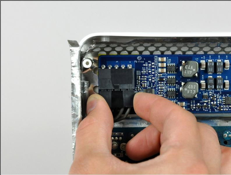
**⚠** This step brings your hands close to the exposed face of the power supply. **Do not** touch the face of the power supply to avoid a high voltage shock from the many large capacitors attached to the board.
