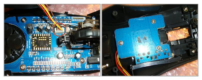
Be gentle when performing this step. Most Kone models have wires connecting the halves of the shell that may be damaged if you yank on them.
