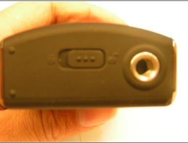
Locate the lock/unlock latch at the bottom of The Flip Ultra HD 2nd Generation and slide it into the unlock position.
