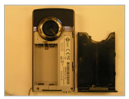
Pull down on the large front cover to to expose the battery slots.
