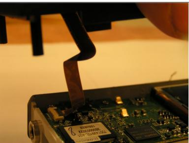
Remove the ribbon cable gently and pull the back cover off
