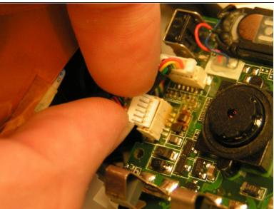
There are two wires with white heads connecting the circuit board to the front of the device. Gently
