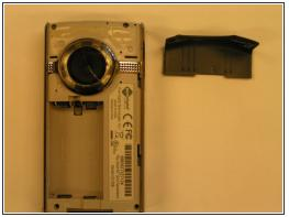
Pry off the top of the camcorder with a flat head screwdriver. The cover is glued on with adhesive so it will take some force to dislodge it from the device.
