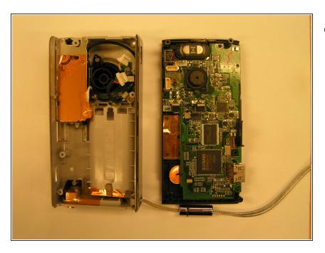
The disassembled Flip Ultra HD
