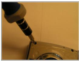
• Use a small Phillips head screwdriver to remove the two screws at the bottom of the battery slot and the two screws above the camera lens.
