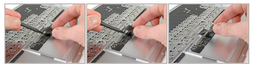
• While carefully lifting the keyboard ribbon cable with one hand, use the tip of a spudger or your fingernail to flip up the retaining flap on the keyboard ribbon cable ZIF socket.
