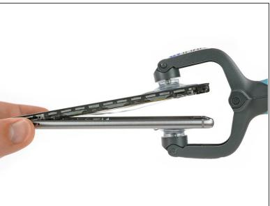
Use an iSclack or a suction handle to separate the display unit from the rear case.
