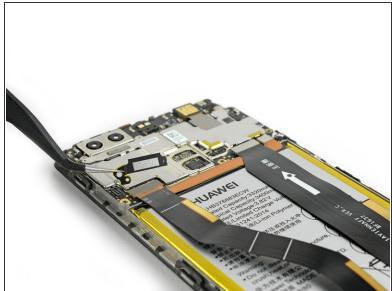
Both metal plates have little hooks. Use a tweezer to free them and unhinge the plates by carefully moving them upwards.
