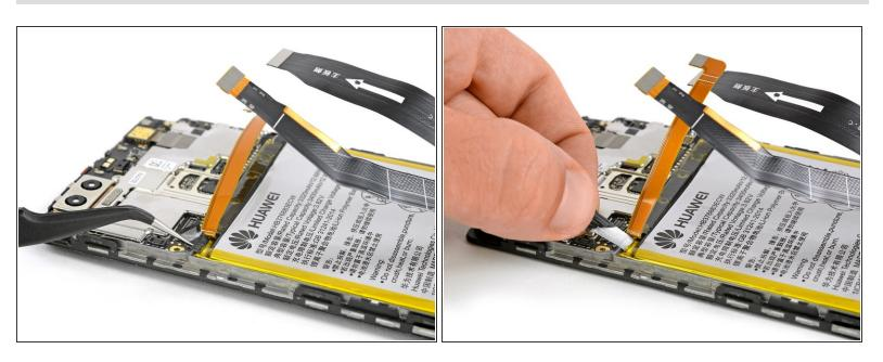
Loosen the end of the other adhesive strip with a tweezer and pull it out. If needed use the iOpener again to soften the glue a little.
