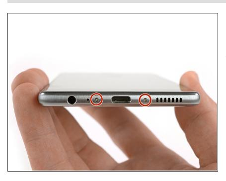
Remove the two P2 Pentalobe screws on either side of the USB C port.
