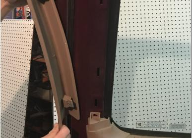
Grasp the door trim panel and squeeze while pulling away from the door until the panel releases.
