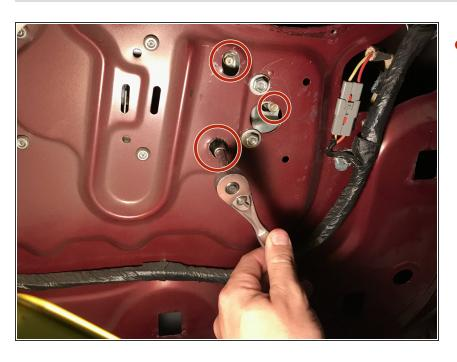
Remove the three bolts holding the window motor with a 8 mm socket.
