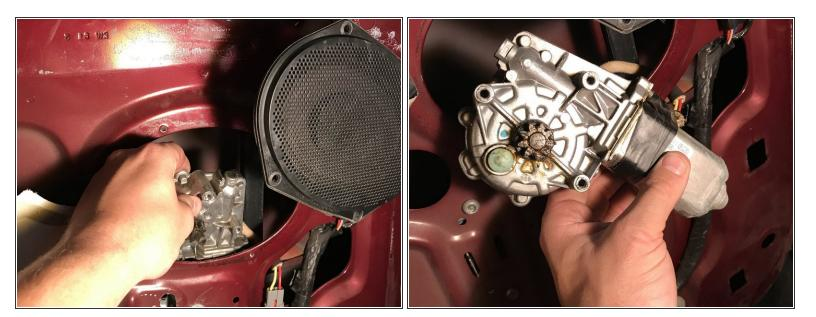
Reach inside the door panel and remove the existing motor.
