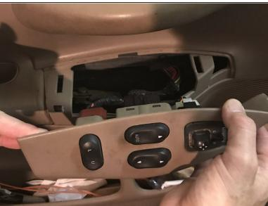
Grasp the window button housing and squeeze while lifting up and away from the door.
