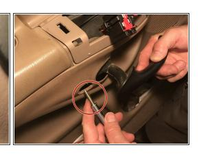
Using a 5/16 nut driver, unscrew the door handle by accessing the bolt inside the door panel.
