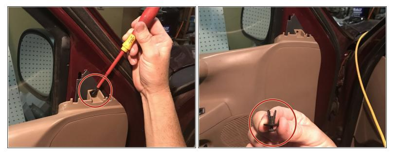
Using a flat head screwdriver, pry off the plastic snap holding the door panel to the door.
