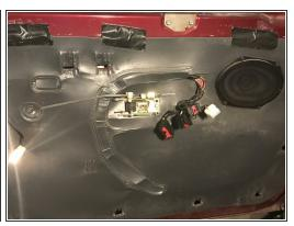
Grab the door panel firmly and lift up and away from the door to release the panel from the door.
