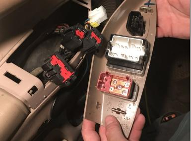
Holding the window button housing, press against the tabs while pulling the plug-in away from the housing. Repeat this for all four control buttons.
