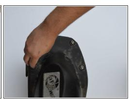
• Remove 6-8mm (5/16") x 25mm hex bolts using the 8mm (5/16") hex key.
