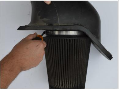
Loosen hose clamp holding air filter to air filter assembly using flathead screwdriver.
