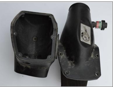
Remove top cover from air filter assembly.
