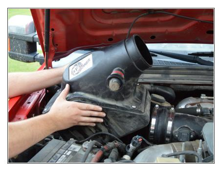
Pull air filter assembly out of vehicle.
