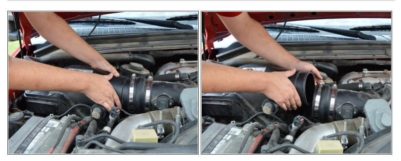
Pull air filter assembly away from silicone tube connector.
