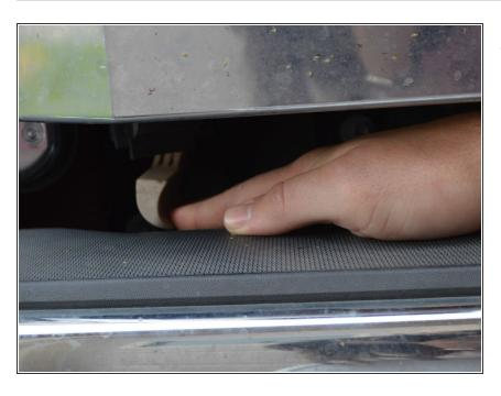
Press the latch located under the grill to unlock hood.
