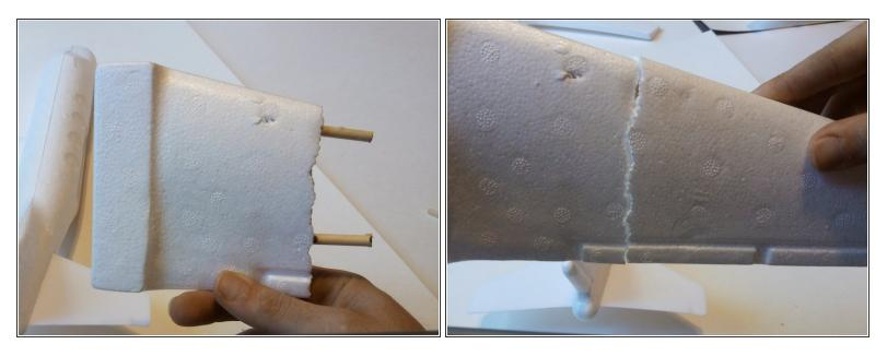
• Insert the dowels back into the holes and bring both parts of the wing back together.
