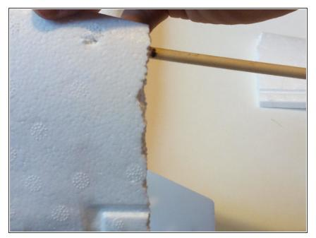
• Once the the dowel piece has been pushed into the interior part of the wing, make a mark where the wood and foam meet.
