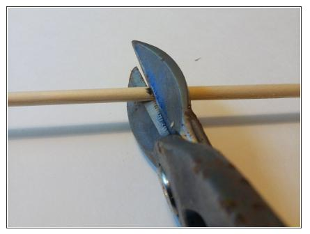
After you have made your 6 inch mark, use a pair of wood snips to cut the dowel cleanly at 6 inches.
