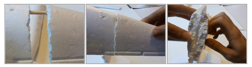
Slide the exterior part of the wing towards the interior part of the wing and dowel, creating a hole in both parts of the wing.
