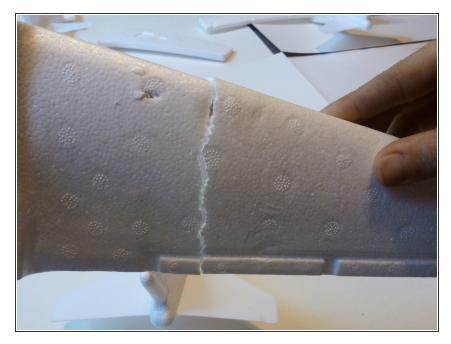
• Follow the same method as step 9 and create a hole in the exterior section of the damaged wing.
