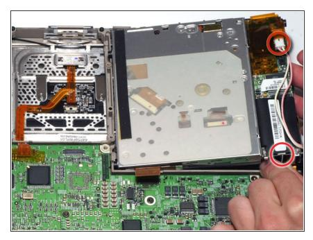
Lift the drive up on the right side so that you can access and disconnect the modem cable and inverter cable.
