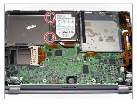
To free the hard drive, remove the two T8 Torx screws from the right wall of the battery housing.
