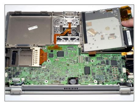
Remove the drive by lifting the right edge up and out of the computer.
