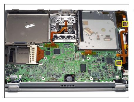
Disconnect and remove the indicated orange ribbon cable.
