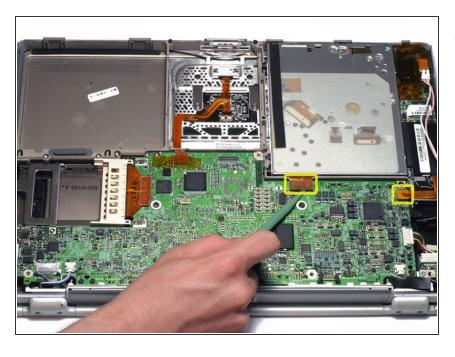
Disconnect the two orange connectors from the logic board, removing tape as necessary.
