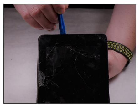
• Using a plastic opening tool, pry open the back cover from the tablet.
