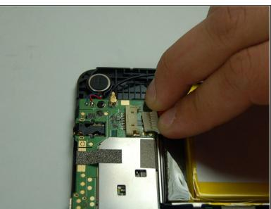
Use a spudger to disconnect the battery from the motherboard.
