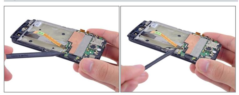
• Using the pointed end of the spudger, pop the antenna cable from its connector on the motherboard.
