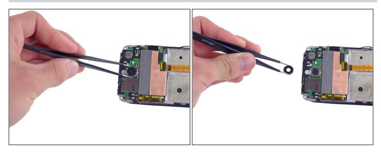
A camera filter is now free to move, so remove it using tweezers.
