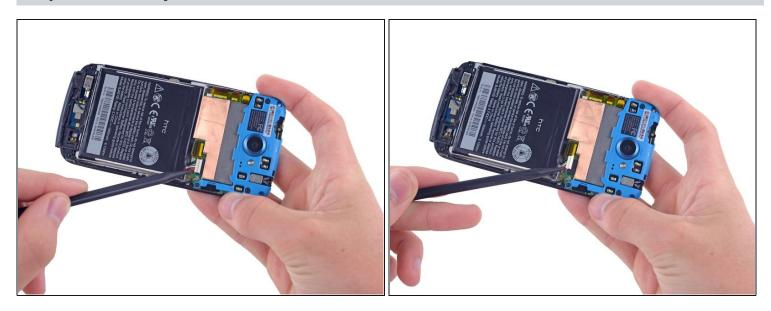
Using the pointed end of a spudger, lift the battery cable and release the connector.
