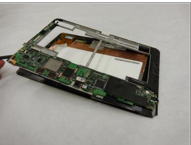
Use a Phillips #00 Screwdriver to remove the 3mm screws that connect the metal board with the screen.
