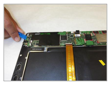
• Remove the motherboard using the plastic opening tool gently.
