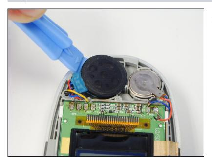
After the solder has been removed, pry out the speaker with the plastic opening tool.
