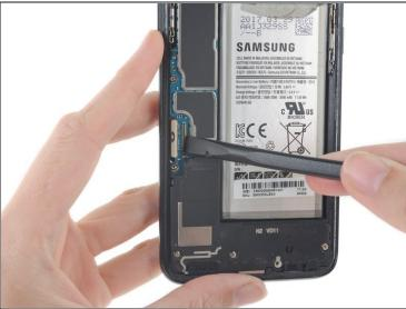
Use the flat end of a spudger to disconnect the display and digitizer connector.
