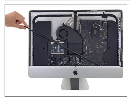
Remove the lower support bracket (a.k.a. "chin strap") from the iMac enclosure.
