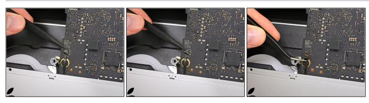
• Flip the latch on the microphone <u>ZIF connector</u> and pull the cable out of its socket on the logic board.
