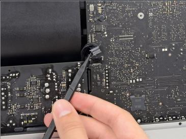
• Use the tip of a spudger to push each side of the power supply control cable connector and gently *walk* it out of its socket.
