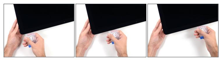
• Slide the card toward the center of the display to cut any of the remaining adhesive along the top right corner of the iMac.
