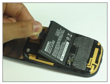
• Carefully pull up on the tab to remove the current battery.
