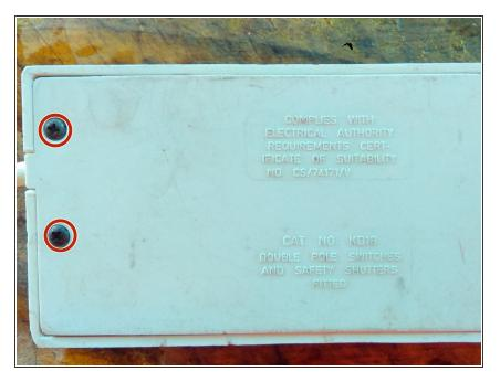
Remove the two screws securing the back plate.
