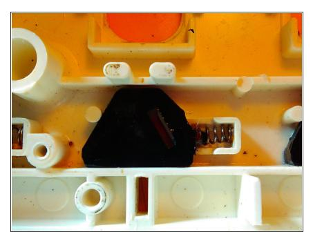
Each cover plate has a small spring, these can be rusty which will prevent the covers moving, thereby preventing the insertion of an appliance plug.
