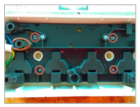
After removing the backplate, remove the four screws that secures the internal assembly to the box.
