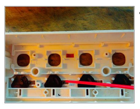
Spray a small amount of WD40 onto the springs, then manipulate the covers until they move freely.
