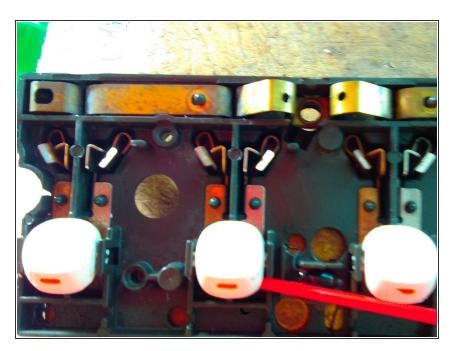
Spray a very small amount of WD40 into the rocker mechanism of each switch. Then manipulate the switches until they move freely.
