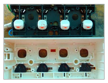
The disassembled powerstrip. The rocker switches are in the section removed from the box. In the box, there are spring-loaded covers where the appliance power plugs are inserted. These covers prevent dirt entering the box.
