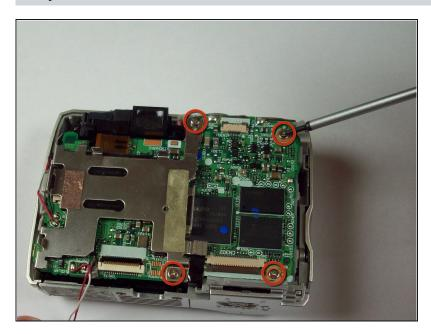
Locate and remove the four 4.25 mm screws on the motherboard using a Phillips 00 screw driver.
