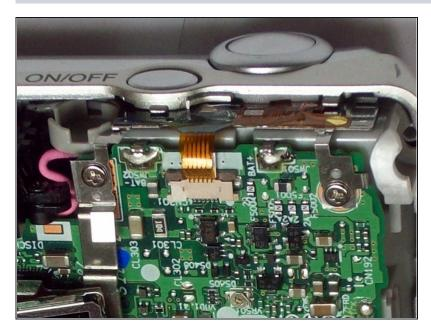
Remove the ribbon cable on the top right of the motherboard. To remove the cable, slide the two grey tabs, located on both sides, towards the top of the camera and gently pull the cable out.
