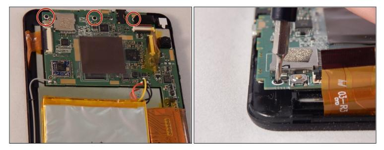
• Remove the three screws that are located at the top of the circuit board with the screwdriver. (2.4 mm head, 3.9 mm in length)
