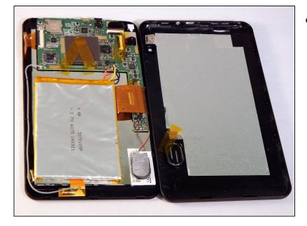
The back panel should now be disconnected from the device. This provides access to the components of the device for repairing and replacing parts of the tablet.
