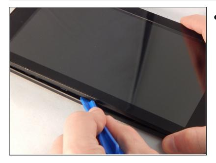
• Begin by inserting the plastic opening tool into the seam between the back and front of the case and carefully pry the back from the front.
