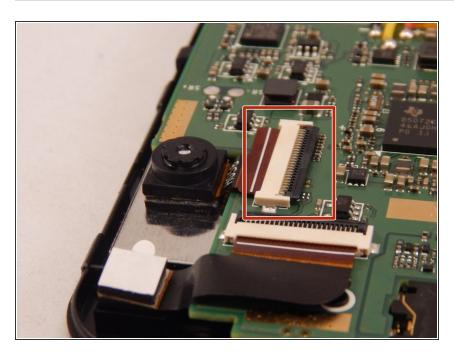
With tweezers, flip the black latch to open the pin connector and remove the cable.
