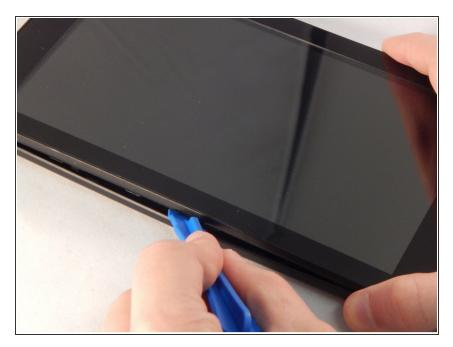
Begin by inserting the plastic opening tool into the seam between the back and front of the case and carefully pry the back from the front.
