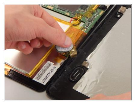
Remove the tape holding the speaker to the back panel.
