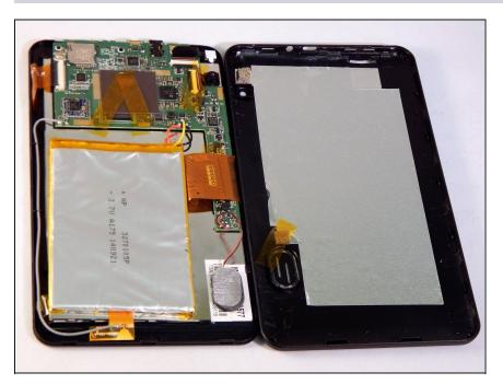
The back panel should now be disconnected from the device.
