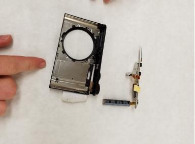
Grab the top of the camera and take it out. Then grab the flash assembly and slide it out.
