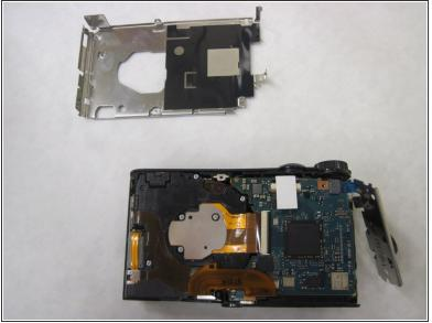
Remove silver Phillips 4 mm screws using the J00 head screwdriver tip from the metal cover. Once done take the metal cover off with your hands.
