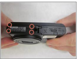
Remove 6 black Phillips 4 mm screws using the J00 head screwdriver tip from the sides and bottom of top cover.
