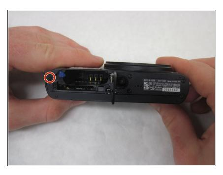
Remove the black Phillips 4 mm screw using the J00 head screwdriver tip from inside the battery inclosure.
