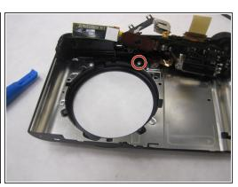
Remove the silver Phillips 4 mm screws using the J00 head screwdriver tip from the metal piece and remove the 4mm screws from the metal piece lining the lens assembly hole.
