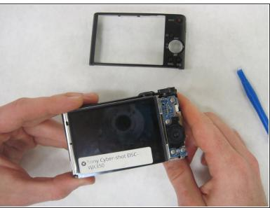
• Use the plastic opening tool to take back cover off. Then take out the LCD screen with your hand.
