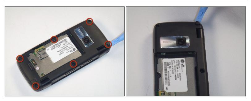
First remove the rubber stoppers covering the screws on the back of the phone by prying them up and away from the phone.
