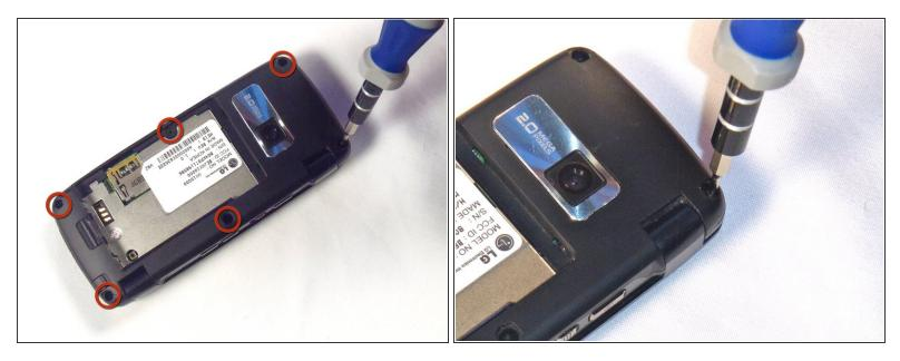
• Remove the 3.61mm length, Phillips screws from the back of the phone using the #00 screwdriver.
