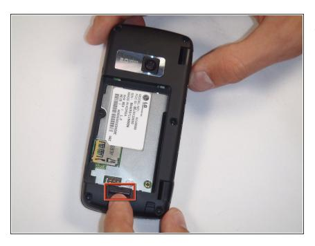
Pull down on the button at the bottom of the phone. The battery will pop up and can then be safely removed.
