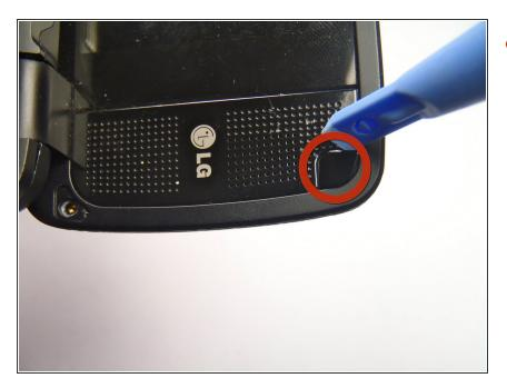
Use a plastic opening tool to pry up and remove the screw covers located in the corners by the speakers
