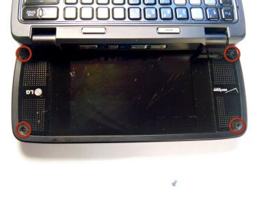
Unscrew the four screws under the covers with a #00 screw driver.
