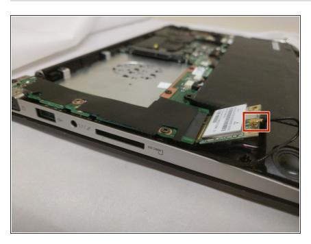
Use precision tweezers to pry the black wire with a gold plug off the main gold plug on the module.
