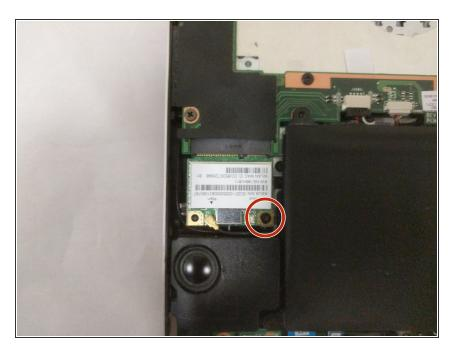
Use a Phillips J0 screwdriver to remove the one black 3mm screw.
