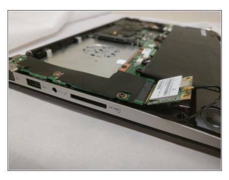
Use an up and away motion to pull the module out of its slot.
