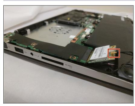
Use precision <u>tweezers</u> to pry the black wire with a gold plug off the main gold plug on the module.
