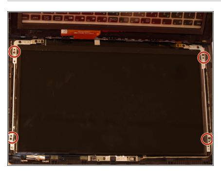
Using a Phillips #0 screwdriver, remove the four 2mm silver screws located at each of the four corners of the screen.
