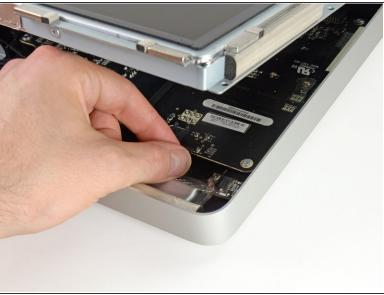
Using your fingers, carefully pull the vertical sync cable out of its socket on the LED driver board near the top left corner of your iMac.
