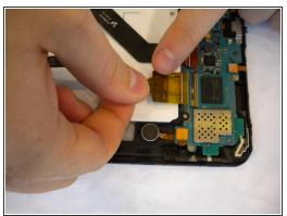
Carefully pull out the yellow flexible ribbon cable to disconnect it from the motherboard.
