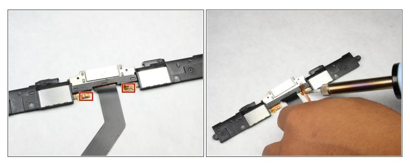
Desolder the two connections to separate the speakers from the charger port.
