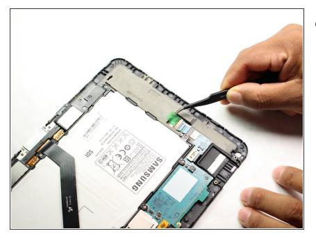
Remove green tape from lcd connector.
