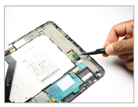
• Pull lcd cable out of connector.
