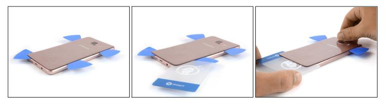
• Insert a <u>plastic card</u> at the bottom and slide it underneath the back cover.
