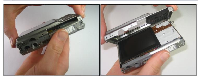
• With the LCD screen facing up towards you, start at the bottom of the camera and gently pull off the back of the casing.
