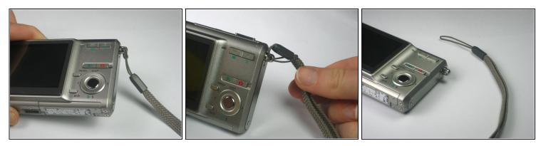
• Remove the strap from the camera by pulling the thin cord out, creating a small loop, then pushing the thicker cord back through this loop.
