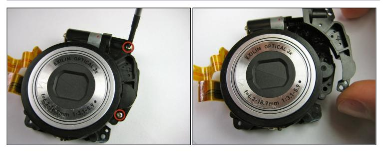
• Now that the lens is fully exposed, remove the two phillips screws (4.34 mm) on front of the lens.
