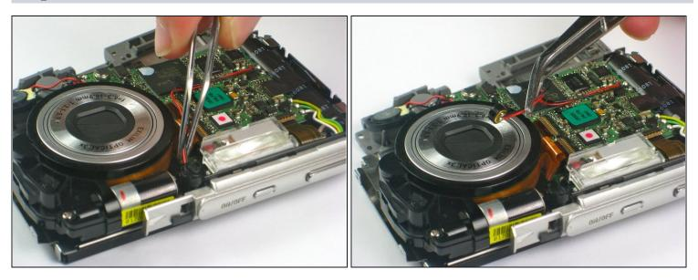
• Use a pair of <u>tweezers</u> to gently move the wire around part of the lens away from it so that you can access the lens.
