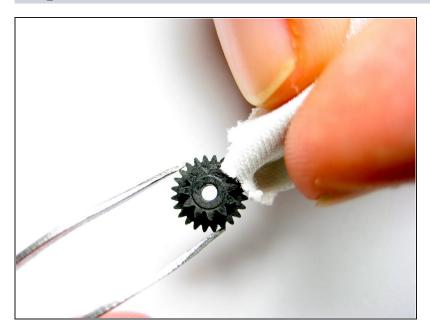
Clean the gear box and the gears with water and a cloth or paper towel. A pin can be useful to dislodge any grit or dirt stuck in between the teeth of the gears.
