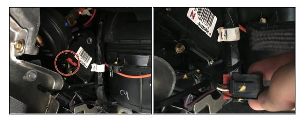
There is a 4-pin cable connecting to the bottom-left of the actuator. There is a tab that can be pressed to release the cable from the actuator.
