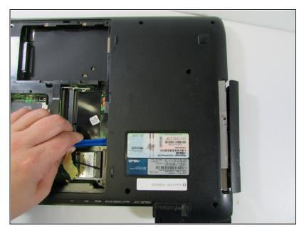
Use the plastic opening tool to push the drive out from the back.
