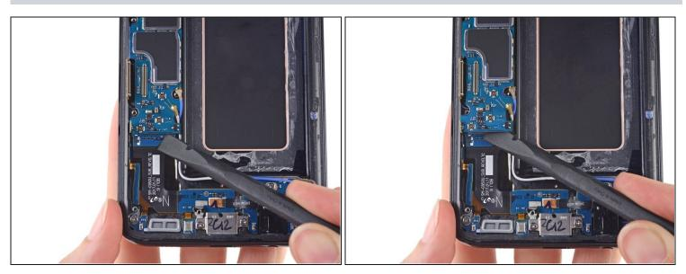
• Use the flat end of a spudger to lift the motherboard and disconnect it from the daughterboard.
