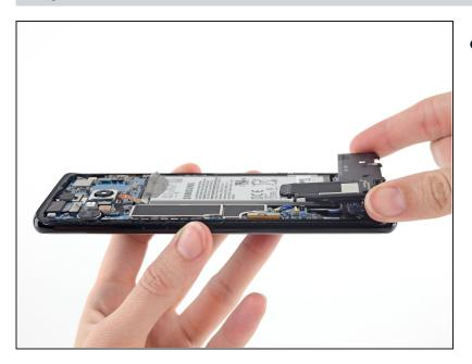
• Remove the loudspeaker assembly.
