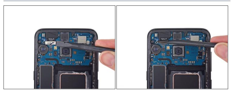
• Use the flat end of a spudger to disconnect the front-facing camera connector.
