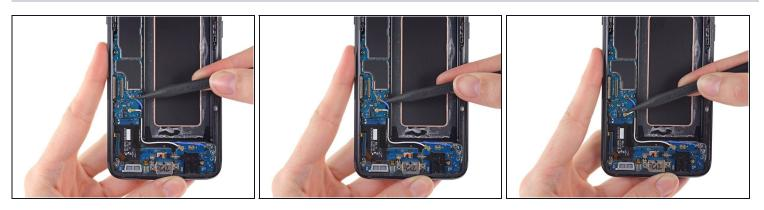
• Use the point of a spudger to disconnect two antenna cables that connect the motherboard to the daughterboard.
