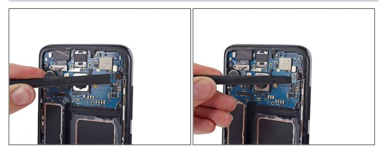
• Use the flat end of a spudger to disconnect the sensor array connector.
