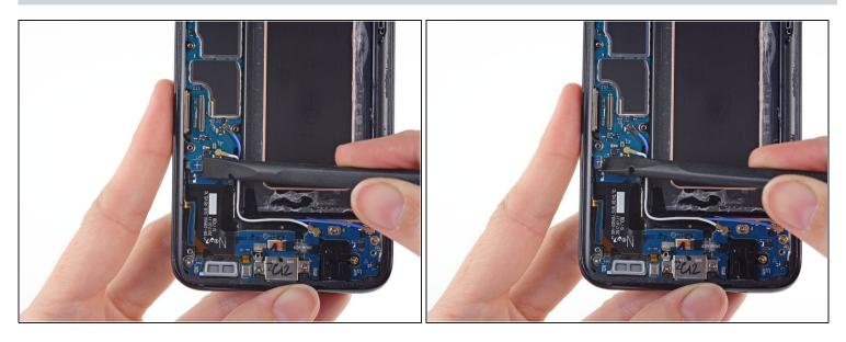
• Use the flat end of a spudger to disconnect an antenna ribbon cable that connects the motherboard to the daughterboard.
