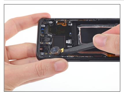
• Use the flat end of a spudger to pry up and remove the vibrator motor.
