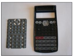
• Peel off the rubber button holder starting in the top left corner.
