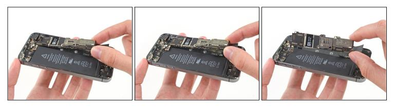
• Pull the logic board slightly away from the rear facing camera.
