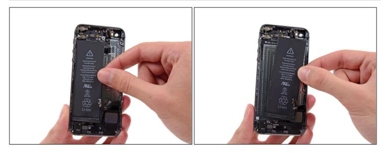
• Remove the battery from the rear case.
