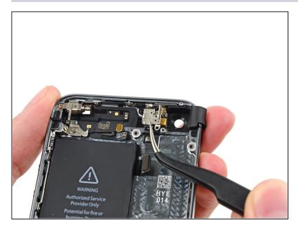
• Remove the rear-facing camera bracket from the rear case.
