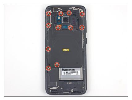
Remove eleven 3.7 mm screws using a Phillips #000 screwdriver.
