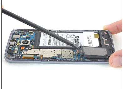
• Use the flat end of a spudger to pry up and remove the loudspeaker assembly.
