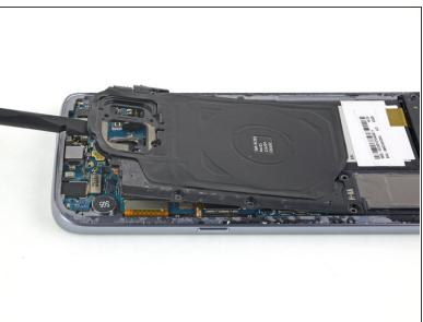
• Use the flat end of a spudger to lift the charging coil assembly out of the phone.
