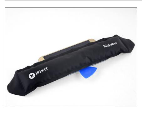
Once the pick is firmly inserted underneath the display, <u>reheat</u> and reapply the iOpener to soften the display adhesive.
