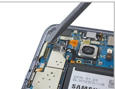
Use the flat end of a spudger to unplug the display and digitizer connector.
