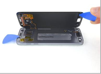
Pry up the side of the display opposite the display cable so that the cable acts like a hinge as the phone opens.
