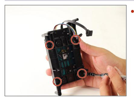
Remove the four black 10mm T10 Torx screws from the black plastic mount.
