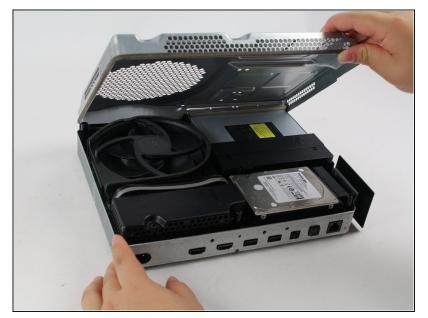
• To access the hardware within the casing, you can pop and lift the top panel of the casing. It should come right off.
