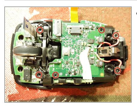
Remove the six screws from the locations circled in red.
