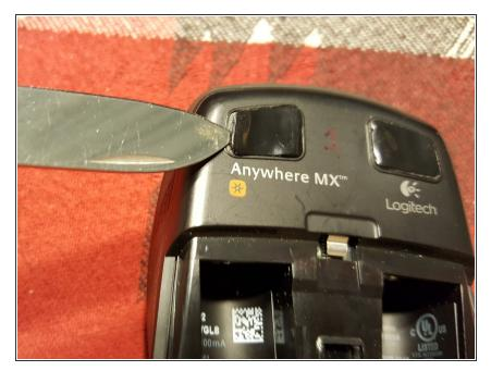
Use the blade to pry beneath the feet of the mouse and remove them.
