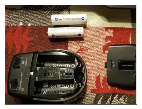
Open the battery cover and remove the batteries.
