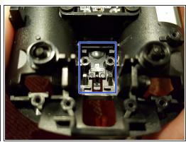
If the plastic piece fell out, this is how it should be positioned when reassembling the mouse. The plastic piece is marked in blue.
