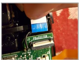
Disconnect the white ribbon cable by flipping the white retention lever up. The ribbon cable should then easily slip out of the unlocked socket.
