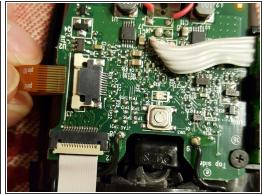
Disconnect the orange ribbon cable by carefully pulling the white locking bar horizontally out from the socket. The ribbon cable should then easily slip out of the unlocked socket.
