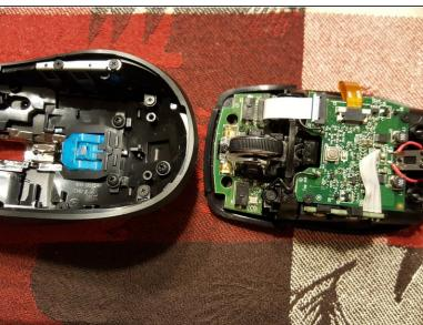
Pry open the mouse using a plastic blade or spudger. The top shell of the mouse should come off relatively easily as there are no clips to disengage between the two halves.
