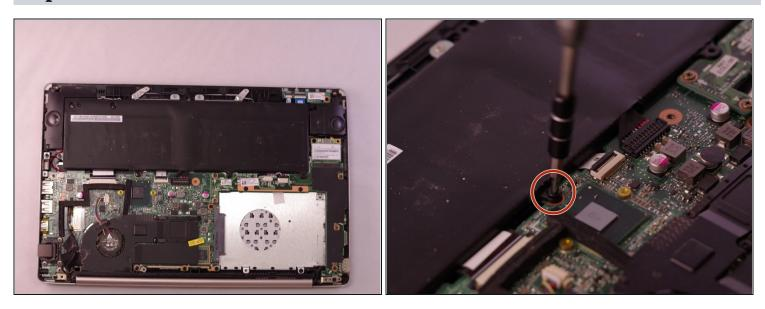
• Using the same Phillips #0 screwdriver, remove the eight black 50mm screws surrounding the battery.
