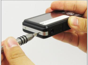
• Remove the two 2 mm silver screws using a Phillips #000 screwdriver.
