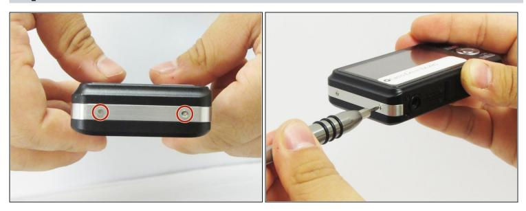
• Remove the two 2 mm silver screws using a Phillips #000 screwdriver.
