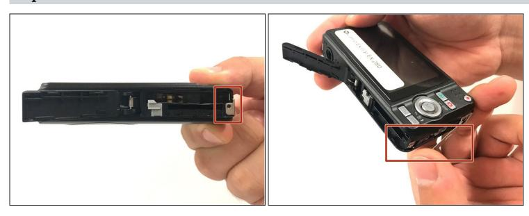
• Carefully remove the silver strip from left side. Open the battery cover and remove the metal strip with fingers by sliding it to the left.
