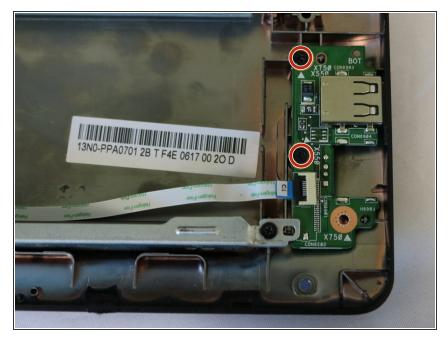
Using a Phillips #0 screwdriver, remove the two 4mm screws holding the port in.
