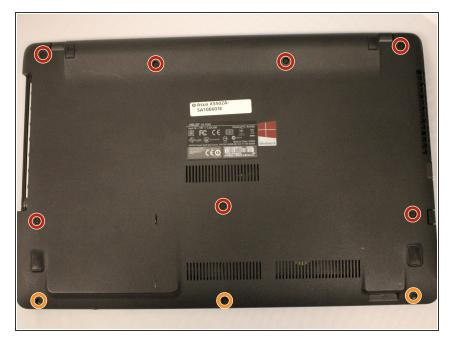
Using the Phillips #0 screwdriver, remove the seven 14 mm screws on the bottom of the laptop.
